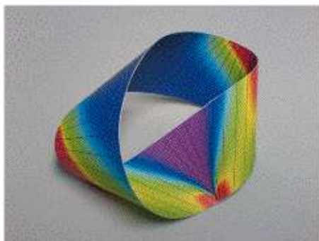
Figure 1 Photo of a paper Möbius strip of aspect ratio 2x. The strip adopts a characteristic shape. Indextensibility of the material causes the surface to be developable. Its straight generators are drawn and the colouring varies according to the bending energy density.
